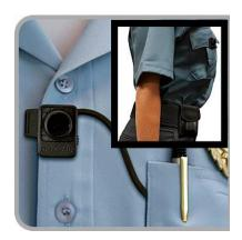
The Digital-Ally FirstVu HD camera is a modular device. The camera is clipped to the officers chest, while the battery and storage fits into the chest pocket of the uniform.
