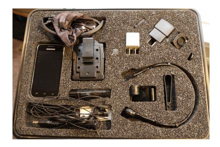
The mounts included are a headband mount, a collar mount, a shirt mount, and a glasses mount. The camera has a small yet very powerful magnet embedded on its side. It marries up with a similar strong magnet in each of the provided mounts. Taser designed the mounts very thoughtfully. The magnet mounts do not move very much, if at all, once it's locked into place. All allow for the camera to be quickly attached at the right angle.
