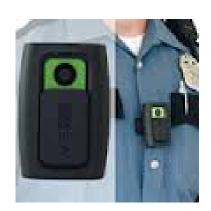
The major operational deficiencies noted for this model is the lack of a pre-event buffer, limited internal storage capacity, short battery life and inability to review video without being tethered to a software equipped computer.
